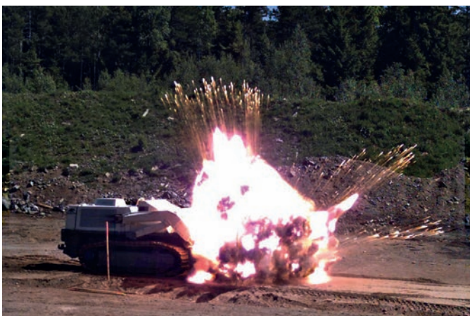
Detonation von 8 kg TNT-Äquivalent. SWEDEC CWA 15044 Certification (2014), Equivalent NATO, STANAG 4569 Level 3 Mine Blast Threat.
