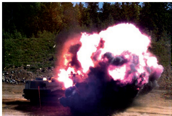
Detonation von 8 kg TNT-Äquivalent. SWEDEC CWA 15044 Certification (2014), Equivalent NATO, STANAG 4569 Level 3 Mine Blast Threat.
